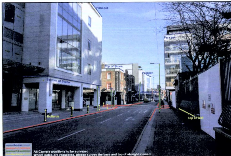
Fig.7: Fixed reference points marked for surveyour.
